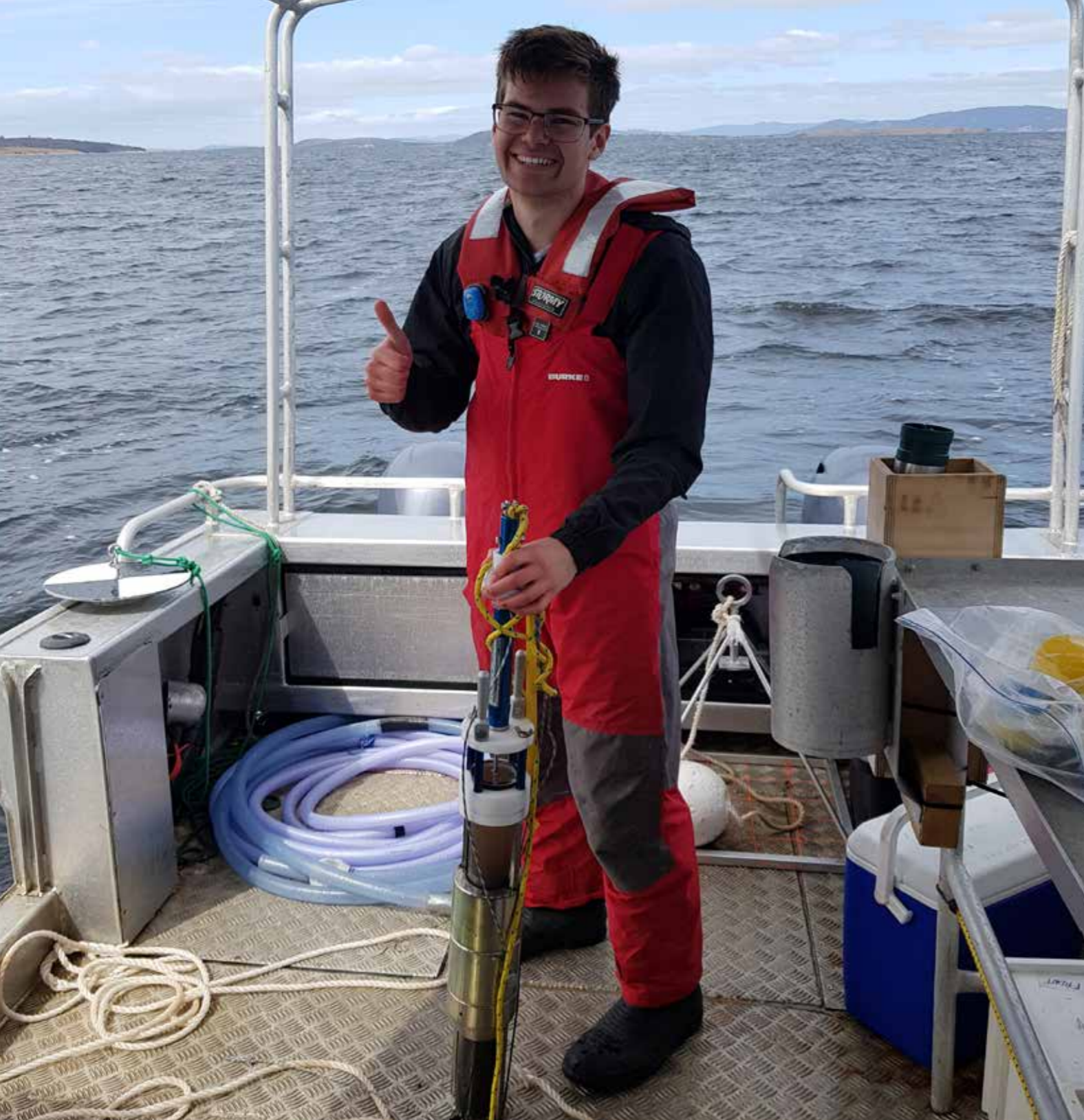
Harrison Stevens, AINSE PGRA Scholar and Ph.D. student at the University of Tasmania, Australia, collecting sediment cores using a Uwitec hammer corer. Please see p22 for further details. Image credit: Harrison Stevens.
