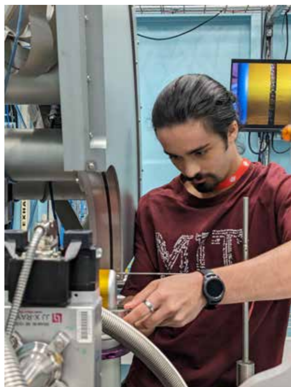
Figure 3: Aligning the cryo-cooler lid on the Powder Diffraction beamline at the Australian Synchrotron for cryogenic temperature X-ray diffraction measurements.
