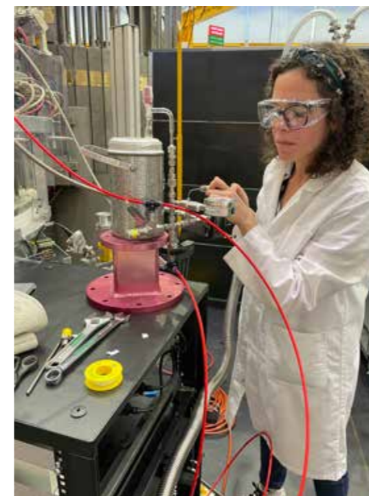
Figure 2: Transfer of synthesised diacetylene to the vanadium can on the WOMBAT neutron diffractometer using the designed gas lines at the Australian Centre for Neutron Scattering (ACNS) in March/2023. Image credit: Helen Maynard-Casely.
