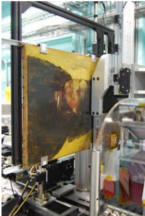
Degas painting being analysed on the XFM beamline at the Australian Synchrotron. Image: David Thurrowgood.
