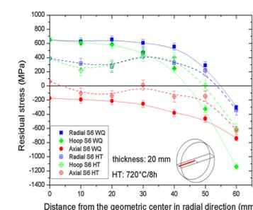
In-Situ Study of the Stress Relaxation During Aging of Nickel-Base Superalloy Forgings, Aba-Perea et al., Metallurgical & Materials transactions A 2019
