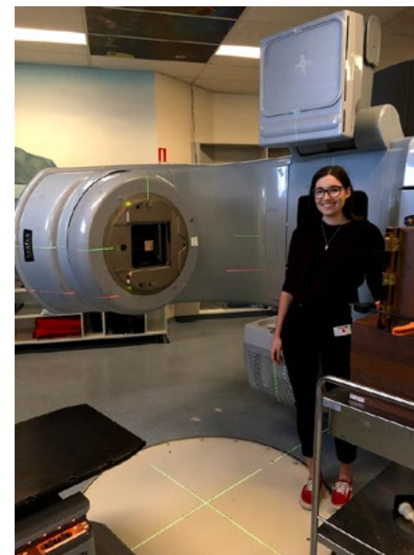
Figure 2 Picture of the Medical Linear Accelerator located at the Illawarra Cancer Care Centre in Wollongong Hospital. The detectors were encased in a solid water-equivalent phantom shown on the right side of the picture to mimic depth within a patient.
