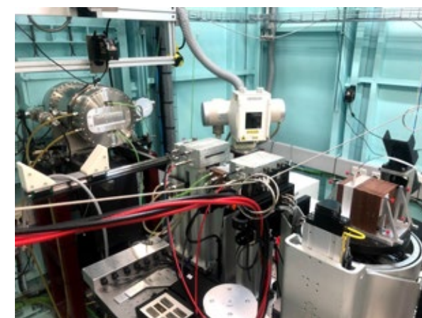
Figure 3: Experimental set-up at the Australian Synchrotron (left) and central microbeams measured using an organic semiconductor exploring their usability to reconstruct the dose profiles for Microbeam Radiation Therapy (right).
