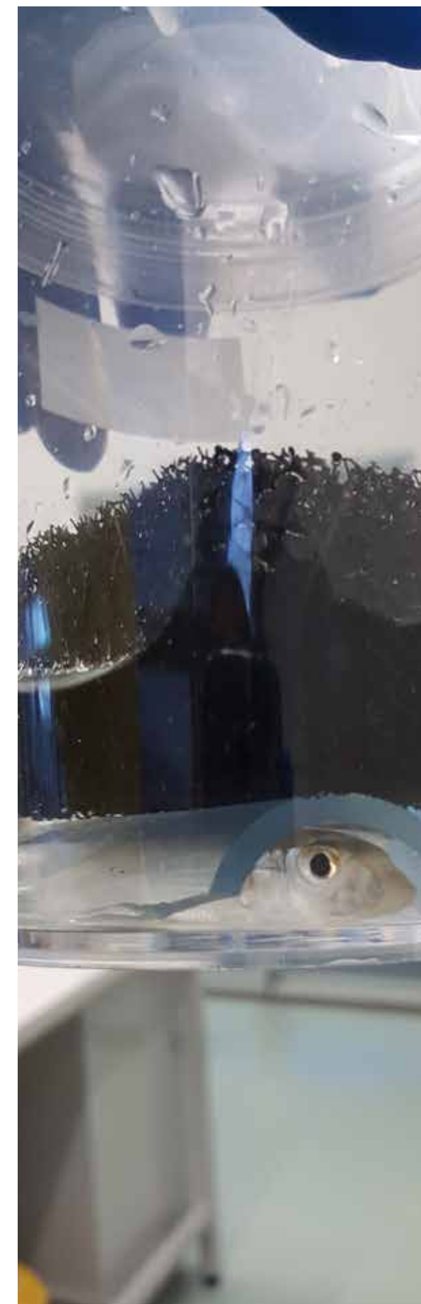
Figure 2: A sand whiting Sillago ciliata in a radioanalysis container, held in a constant position for gamma counting by a semi-circular tube and sponge.
