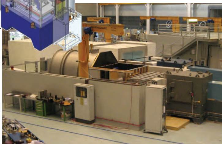
Schematic of Platypus reflectometer and photograph of instrument
