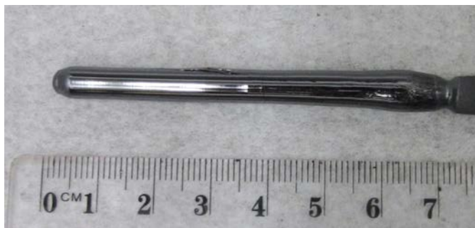
Figure 2 A single crystal of Ca_2FeCoO_5 grown by the optical floating-zone method.
