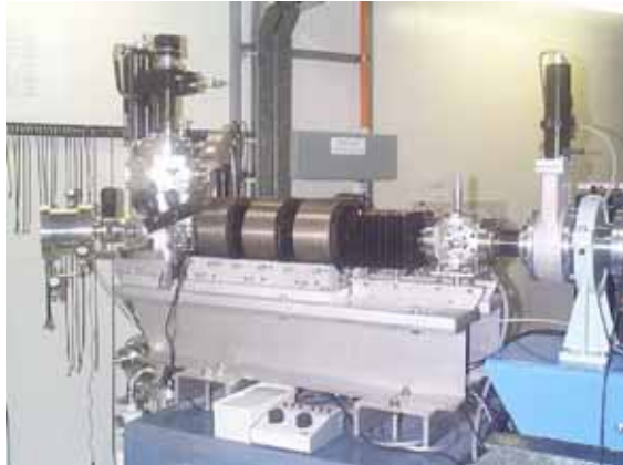
Figure. 3. The current high energy , heavy ion microprobe at ANSTO available to AINSE users. It produces spot sizes down to 5 \mu\text{m} for ions such as p, \alpha , C, Cl, and I.
