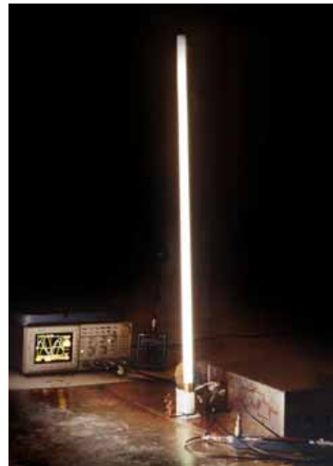
Figure 4: Prototype plasma antenna constructed with fluorescent tube.
