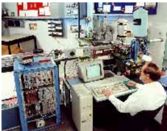
Figure. 2. The current IBA set up on the 3 MV Van de Graaff accelerator. It has 4 simultaneous legs for PIXE, PIGME, FRS and RBS analysis.
