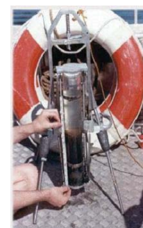
The collection and careful sectioning of aquatic sediments allows us to obtain sediment depth profiles. Profile information includes sediment dates, and concentrations of selenium in the sediments and surrounding porewaters.
