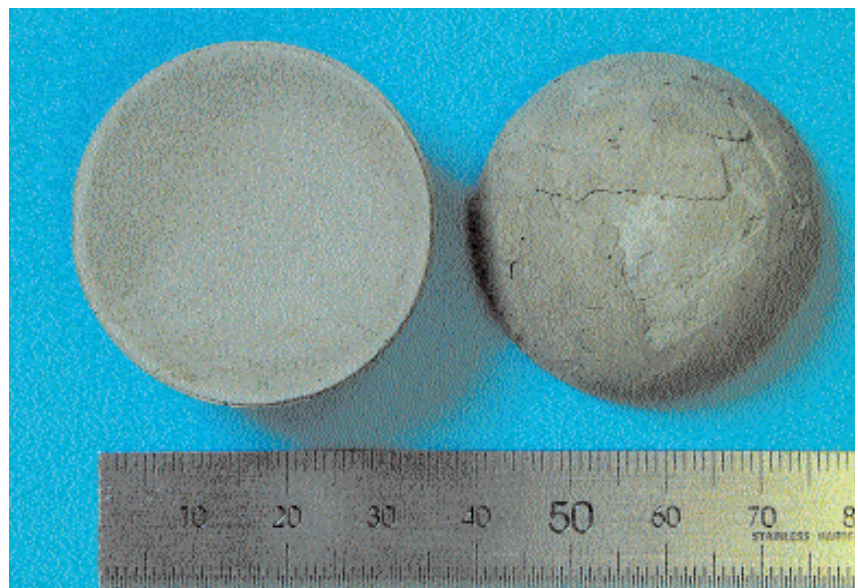
Left: inside the cement sphere the pale rim is related to leaching.
