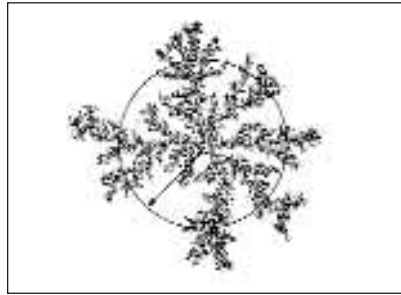
Aluminosilicate fractal cluster whose morphology and structure can be modelled and characterised from data obtained from small angle neutron scattering
