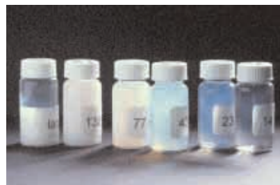
As the particle size decreases left to right, so does the light scattering. All the samples contain 1% polymer, poly(methylmethacrylate) - the perspex polymer. The surfactant used in their preparation ranged from 0-9 mM.
