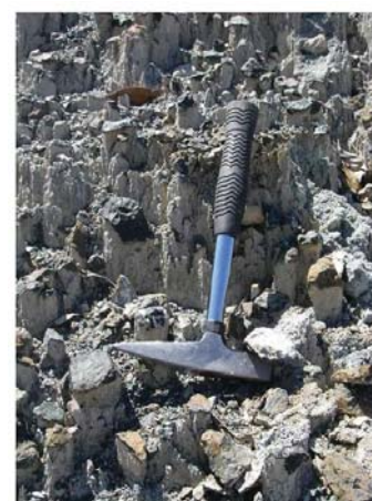
Crust of hydrated magnesium carbonates on mine tailings of Woodsreef Asbestos Mine Image Source: Hans Oskierski
