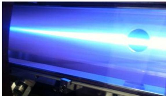
**Figure 1: Argon plasma in the MAGPIE device showing magnetic compression of the plasma which produces high density and high heat flux**
