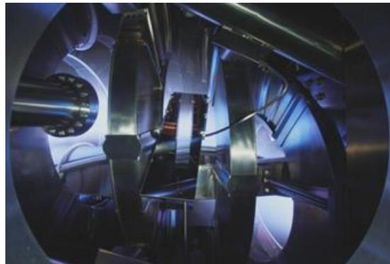
**Figure 2: Plasma in the H-1 Helic. The vertical toroidal coils confine the plasma, and the horizontal ring coil creates the helical twist.**
