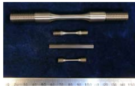
Mechanical testing specimens in descending order: Standard fatigue specimen; miniature fatigue specimen; Young's modulus impulse excitation specimen and miniature creep specimen.
