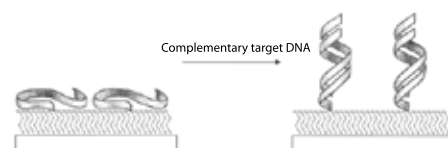
A schematic diagram for the proposed behaviour of DNA end-immobilised on gold for the single-stranded (a) and hybridised (b) DNA-modified substrates
